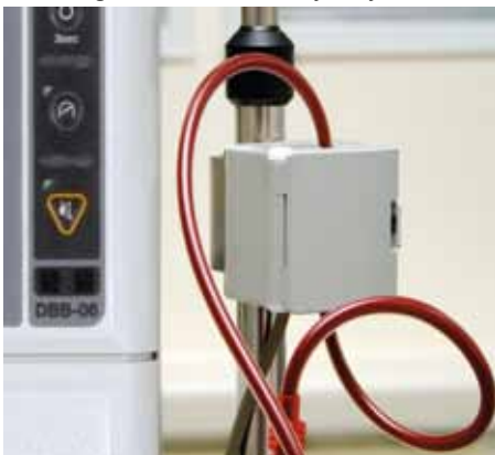
Measuring chamber on the dialysis system
